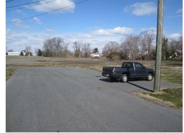
Bioretention systems can be installed in the turfgrass area on either side of the town hall entrance on the southeast side of the building. A strip of parking spaces can be replaced with pervious pavement along the northwest side of the building to capture and infiltrate stormwater runoff from the parking lot. A preliminary soil assessment suggests that the soils have suitable drainage characteristics for green infrastructure.
