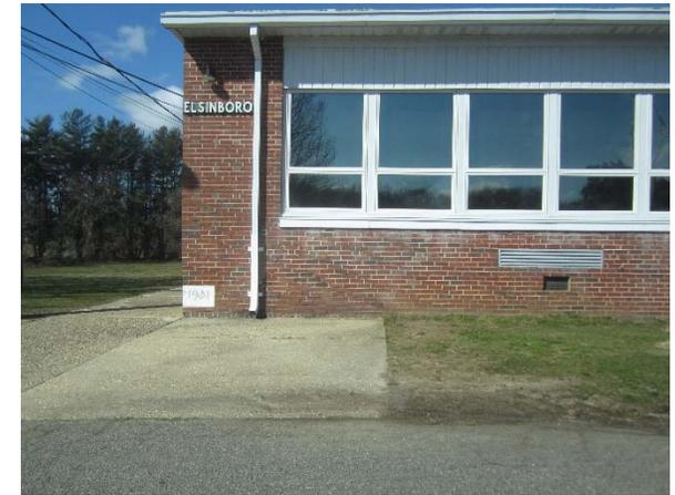
A bioretention system at the southwest corner of the building could capture, treat, and infiltrate rooftop runoff. Two strips of parking spaces in the parking lot can be replaced with pervious pavement to allow stormwater runoff to infiltrate the ground. A preliminary soil assessment suggests that more soil testing would be required before determining the soil's suitability for green infrastructure.
