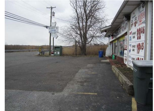
A strip of parking spaces on the east side of the building can be replaced with pervious pavement to capture and infiltrate stormwater. A preliminary soil assessment suggests that more soil testing would be required before determining the soil's suitability for green infrastructure.
