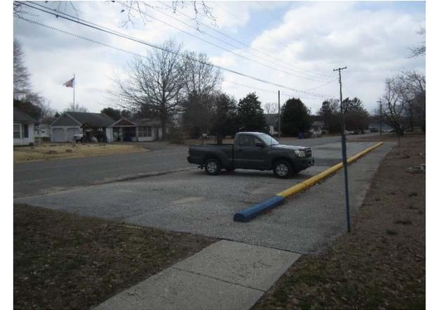
A bioretention system can be installed at the southwest corner of the building by redirecting downspouts to capture rooftop runoff. A strip of parking spaces to the west side of the building can be replaced with pervious pavement to capture and infiltrate stormwater. A preliminary soil assessment suggests that the soils have suitable drainage characteristics for green infrastructure.
